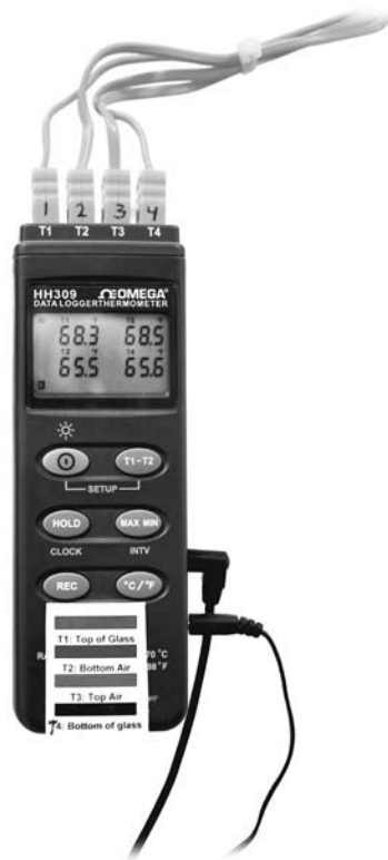
FIGURE 2: SOME PYROMETERS CAN RECORD DATA.
