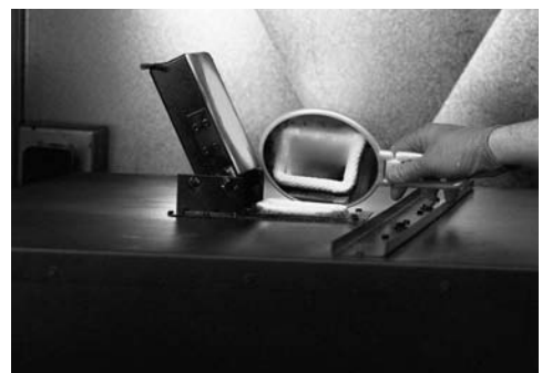
FIGURE 7: USING A MIRROR TO CHECK FOR CONDENSATION.
