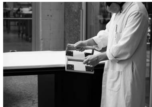
FIGURE 9: SANDING THE SHELF USING A LARGE SANDING BLOCK.
