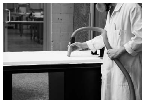
FIGURE 10: VACUUMING DUST FROM THE SHELF AFTER SANDING.
