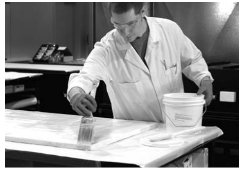
FIGURE 8: BRUSHING QF-180 ONTO THE FIBERBOARD SHELF.
